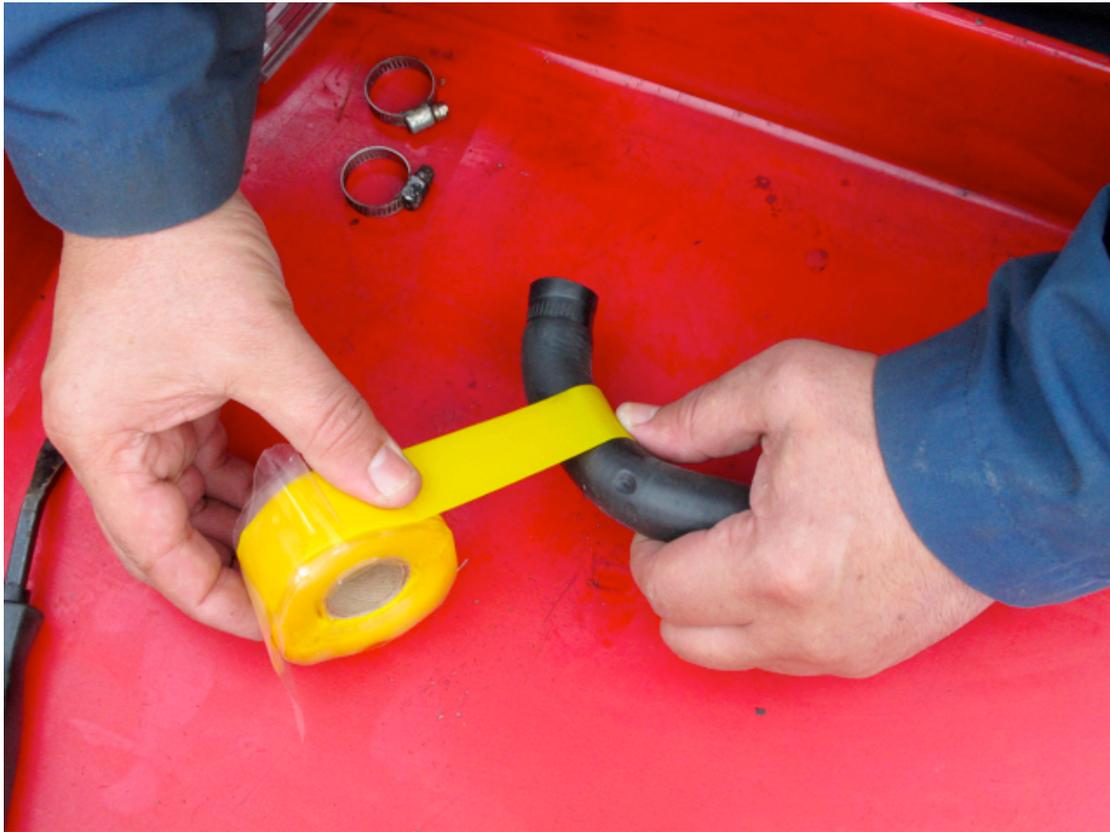
This self-fusing tape has a wide range of applications. Its main attraction is that it's suited for a marine environment. Vinyl tape simply does not work on wet surfaces. It will fall off
